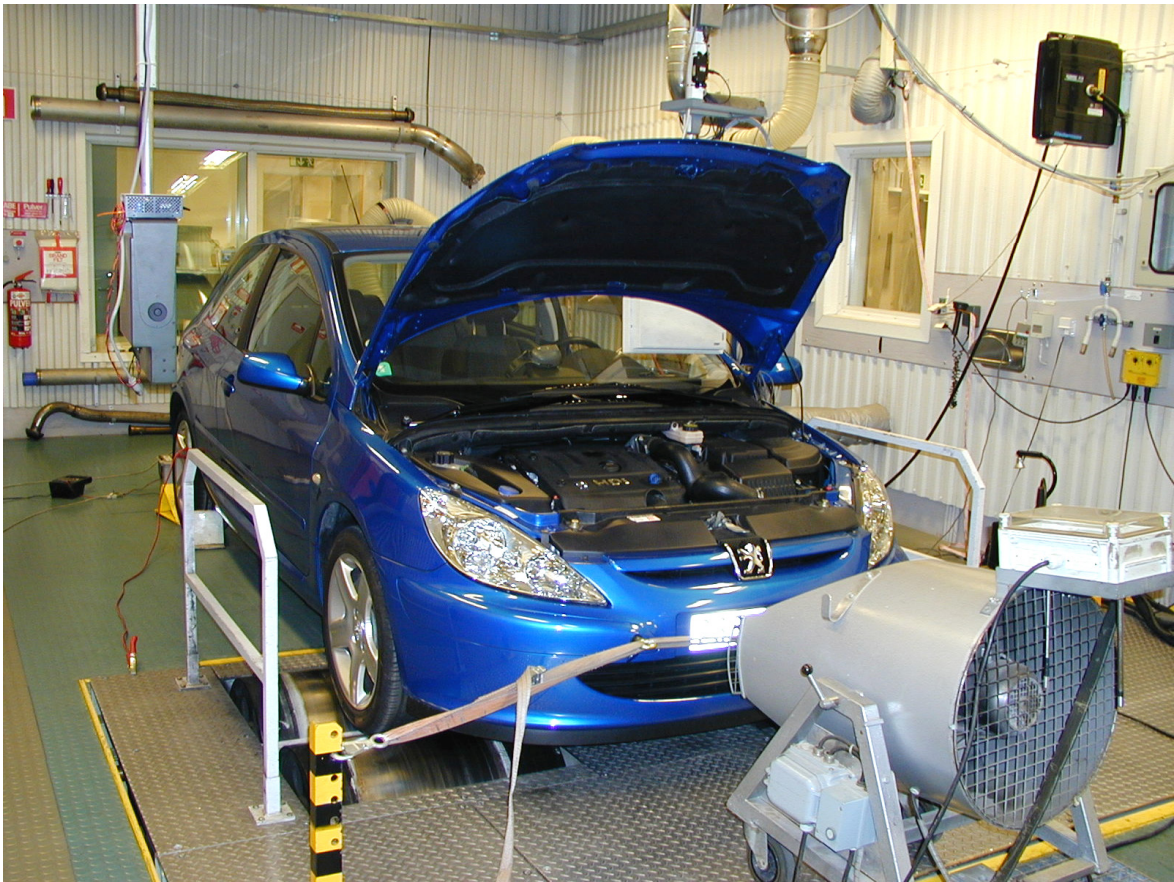
Figure 1. Testing of the Peugeot HDi in the emission test cell at MTC (courtesy of MTC)
